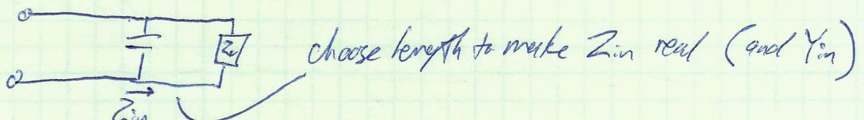
With shunt elements, it is easiest to work in admittance
